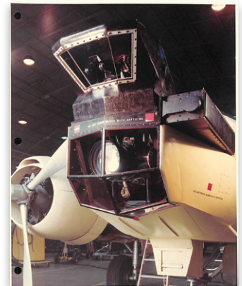
Prototype Laser Target Recognition System (LTRS) installed in the nose of the Hughes Aircraft-owned former B-26B Army serial 44-34538, civil registration N6839D, January 1969.
